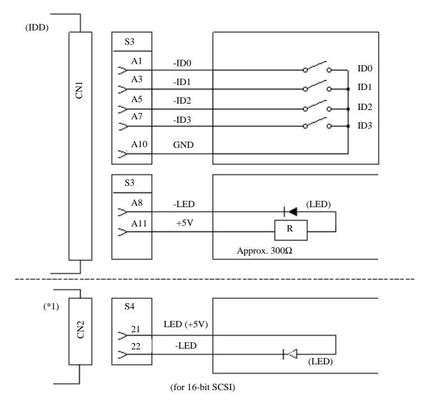
(\*1) For connecting the external LED to CN2.
